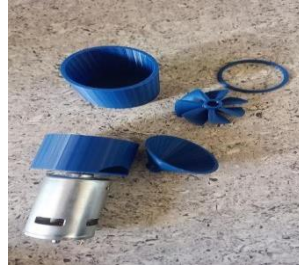
Fig. 3. Fabrication components ready for assembly
