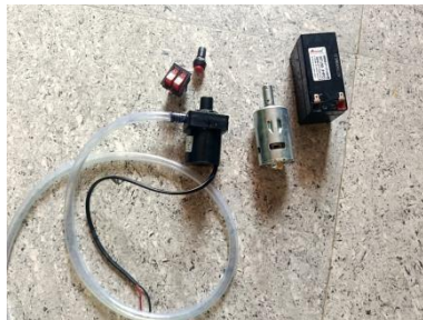
Fig. 2. System components and materials used for assembly
